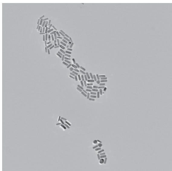
Fig. 3. TEM image of gold NRs of AR 3.5 \pm 1 used for the growth of gold nanowire; the scale bar is 100 nm.
