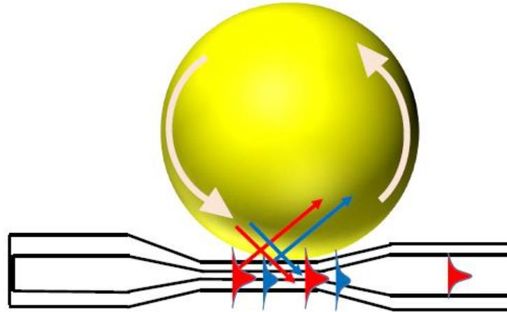
Fig. 1. Coupling of two fiber modes to a single microresonator WGM.
