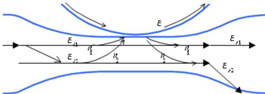
Fig. 2. Two input modes coupling to a single microresonator mode.
